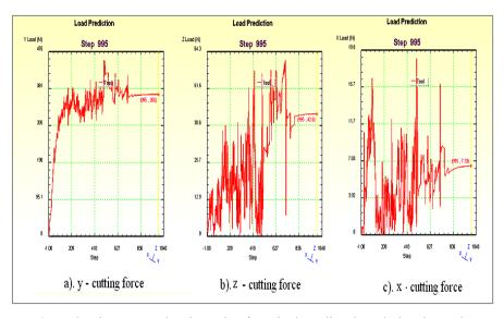
Figure 8 The generated main cutting force in three directions during the cutting simulation processes (rake angle of + 15 deg, cutting speed of 100 m/min, feed rate of 0.35 mm/rev and DOC of 0.3 mm. a) y-cutting force, b) z-cutting force, and c) x-cutting force.
