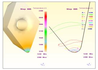
Figure 7 Generated temperature on the edge of carbide cutting tool for rake angle of + 15 deg, cutting speed of 100 m/min, feed rate of 0.35 mm/rev and DOC of 0.3 mm.
