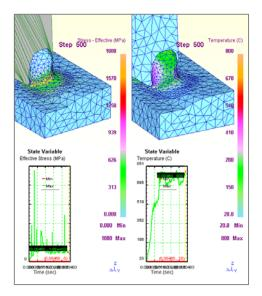
**Figure 4** Example of the transient simulation result for the cutting speed of 100 m/min and rake angle of +5 deg (after running in 500 steps).
