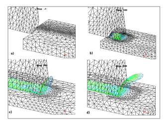
**Figure 3** (a) Initial mesh and tool indentation, (b) Chip formation at step 100,(c) Chip formation at step 300, (d) Developed continues chip at step 500.
