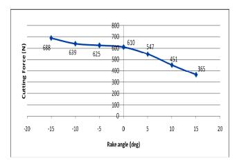
**Figure 9** The cutting force at the edge of carbide cutting tool in various rake angles of +15, +10, +5 deg (positive section), 0 deg, and rake angle of - 5, -10, and -15 deg (negative section).
