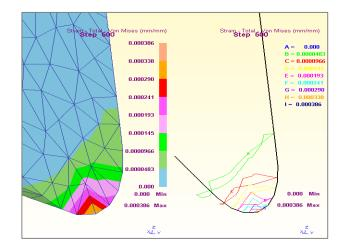
Figure 6 Total Von Misses strain at the edge of carbide cutting tool for rake angle of +15 deg, cutting speed of 100 m/min, feed rate of 0.35 mm/rev and DOC of 0.3 mm.
