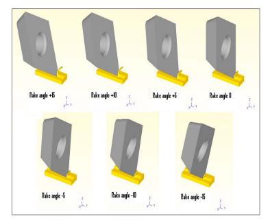
**Figure 2** Various set up of rake angles in positive section (+15,+10, and +5 deg, 0 deg, and negative section (-5, -10, and -15 deg).
