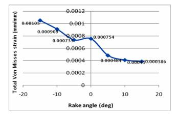
**Figure 11** The total Von Misses strain on cutting edge in positive rake angle (+15, +10, and +5 deg), 0 deg, and negative rake angle (-5, -10, and -15 deg).
