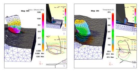
Figure 14 Effective stress in work for the rake angle of +15 deg, cutting speed of 100 m/min, feed rate of 0.35 mm/rev and depth of cut of 0.3 mm.
